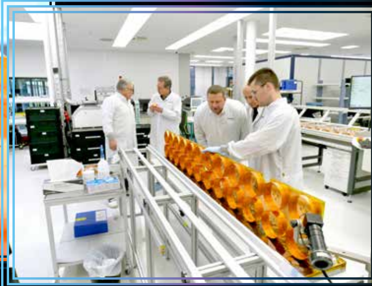
Fully-assembled subarray with 24 ring structures
