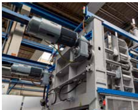
Fast drive types for CoreLess technology, shown here: Kurtz POLY FOAMER with electric drives
