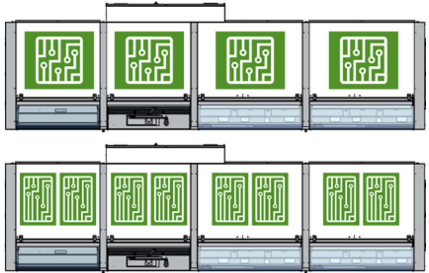
Top: 4 PCBs with max. 610 x 508 mm in the VERSAFLOW ONE XX (3 PCBs with ONE X version); bottom: 8 PCBs with max. 350 x 508 mm in the ONE XX with second stopper (6 PCBs with ONE X)
