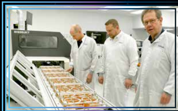
2.4 m long product carrier, milled from a single piece and fitted with an assembly
